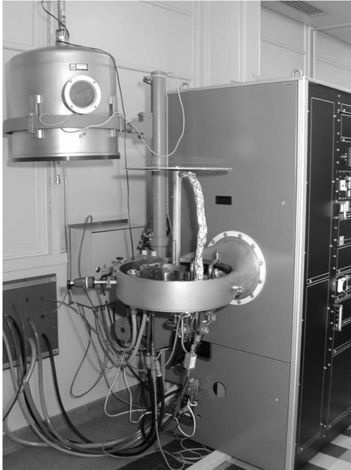
Figure 5.9: View on the evaporator clock of the Univex 450 system used for the deposition of alignment layers.
