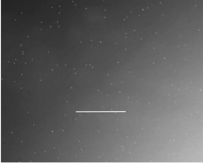
Figure 6.2: Micrograph of the spacer distribution inside the active matrix. The white bar is 200 \mu\text{m} long.
