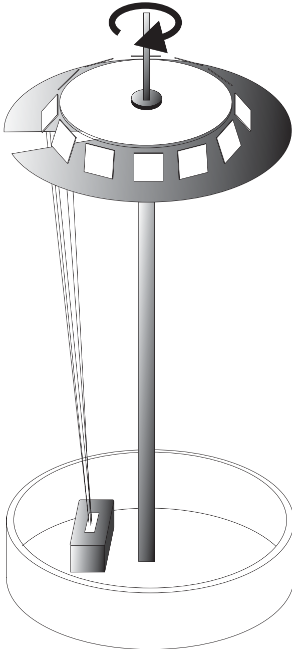
Figure 5.8: Arrangement inside the evaporator. Dimensions are as follows: source to substrates 430 mm, source to shutter 400 mm, diameter of clock 450 mm, diameter of substrate holder 220 mm, shutter opening at the rim 30 mm.
