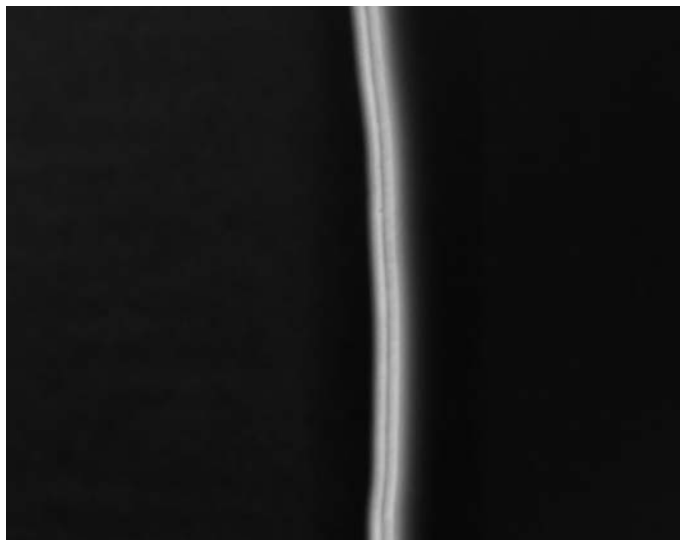
Figure 6.13: Misalignment zone at the interface between the sealing ring and the liquid crystal due to insufficient curing. Left is seal material, right liquid crystal. Photographed through crossed polarisers.
